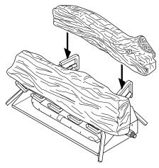
Figure 19 - Installing Front and Back Logs
